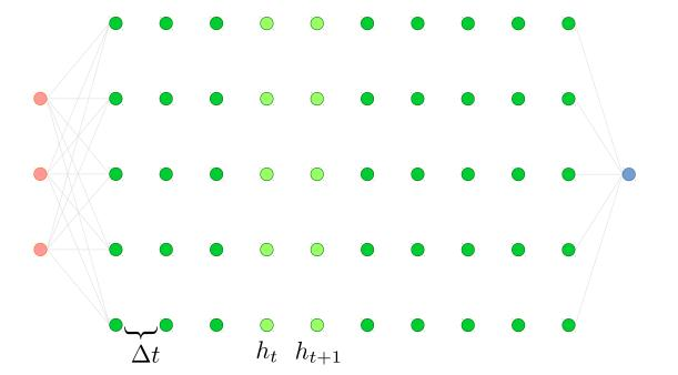
Neural Networks (NNs) layer-to-layer function  $h_{t+1} = F(h_t, w)$
